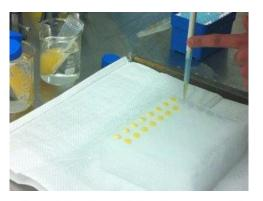
Plunge straws or pellets into liquid N (-196°C)
