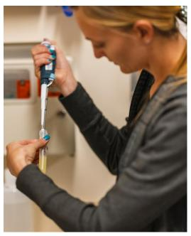
Calibrated pipettor for accurately measuring and slowly diluting semen
