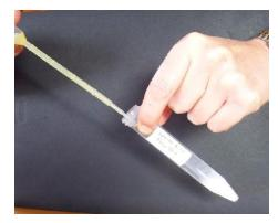
Plastic pipettor for diluting semen with extender: not accurate
