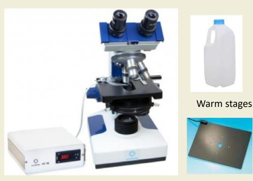
Basic light microscope with X100, X400and X1000 objectives and built in warm stage
