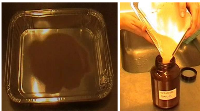
Fig 3. When the contaminated sand is dry, put the TNT sand in an amber glass jar and put the lid on.
