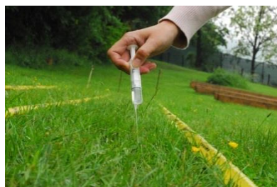
Fig 17. Pour out the TNT water, in different type of terrains, with a syringe. Make sure that it doesn't lie on top of the grass.
