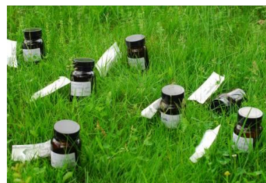
Amber jar with distractors/backgrounds and TNT water in different concentrations.
