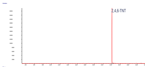
Fig 8. The ERCs in the air above an AP mine, buried in sand at 10 cm depth.
