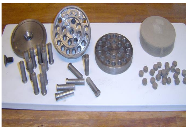
Fig 28b. Tools for producing the soil pellets.
