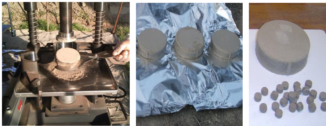
Fig 26 Soil puck and pellets, containing purified TNT water and local soil, produced under high pressure
