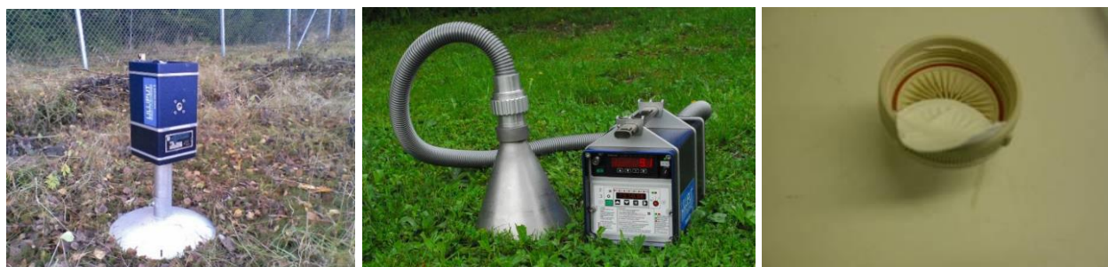
Fig 42. Air samples are collected by using a funnel, a filter and an air pump.
