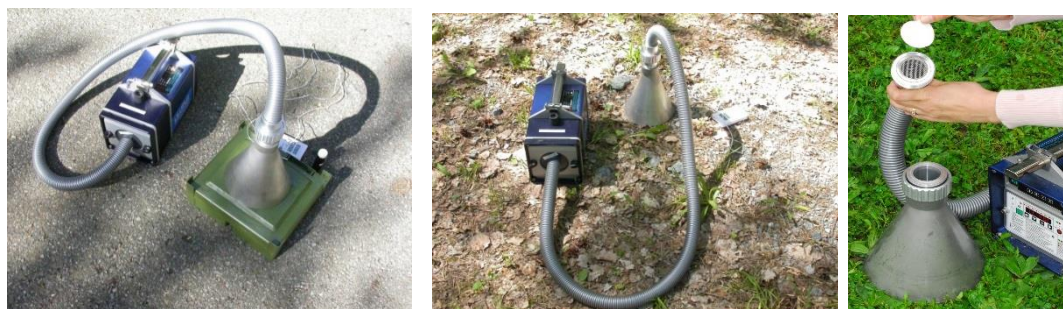
Fig 33. Air samples over different types of mines shows different explosive related signatures
