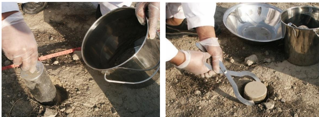
Fig 27 Soil is removed, the puck is produced and the puck is placed back where the soil was taken.
