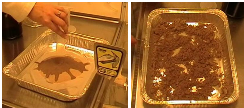
Fig. 2 Pour out the TNT water, and stir until all of the sand is moist.
